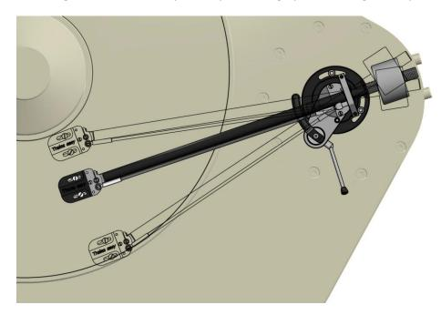
The clever arrangement of six bearing points creates three null points for the horizontal tracking error, plus a zero point for the variable offset angle as well, which is a really novel for a tonearm design. This means the cartridge is guided along the ideal tracing line like that of a parallel tracking tonearm. This reduces side forces tremendously and is audible when listening to the EASY.
